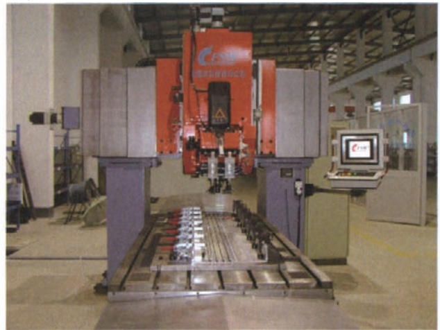
图11 中国首台列车铝合金型材结构产品搅拌摩擦焊设备 Fig.11 Friction stir welding equipment for first train extrusion production in China
